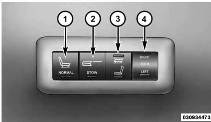
Rear Panel Power Switch Bank
