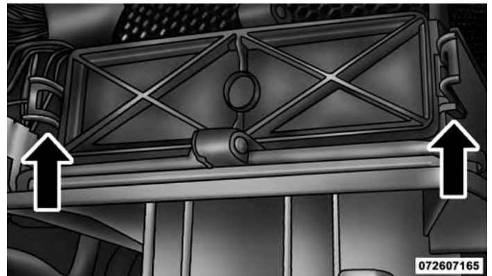
A/C Air Filter Replacement
