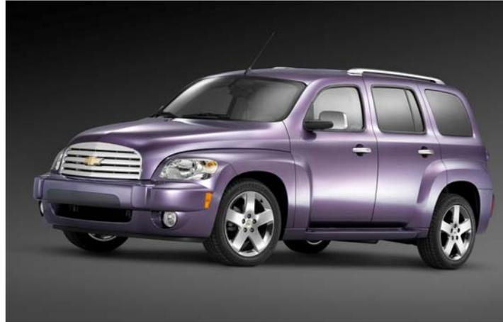
The styling of the HHR was inspired by the sporty Chevrolet SSR and the 1949 Suburban. Built on a Cobalt platform, the HHR is a multi-segment vehicle whose direct competitor is the Chrysler PT Cruiser. It is longer, wider, and has a longer wheelbase than the Chrysler, while the height is roughly the same. The LS version comes equipped with a four cylinder, 2.2 litre engine, while the LT's engine is 2.4 litres.
